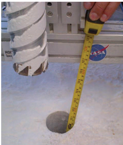
Figure 6 The drill deployed in the field with the extracted cores (top) and drilled hole close-up (bottom)
